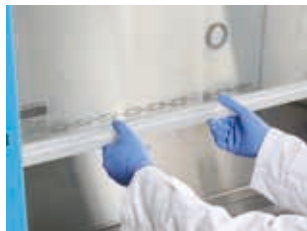
Safety Height-Zone Alarm Function (Alarm sound over 200mm height).
